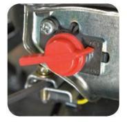
1. Turn engine/motor to Off position.
