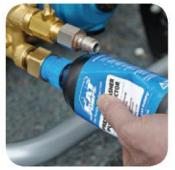
Squeeze bottle to inject pump protector fluid into pump.
